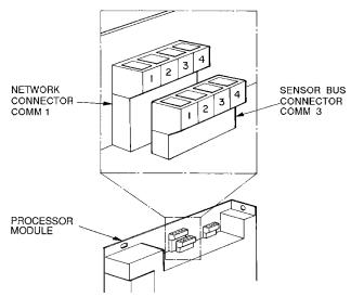
Fig. 24 — Carrier Comfort Network Communication Bus Wiring
